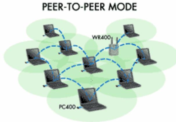
Figure 6: Example of a ad-hoc Peer-to-Peer network.
