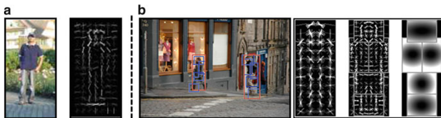
Fig. 1 (a) A sample positive image and its HOG descriptor. (b) Left : detections obtained using part-based human detector in [6]. Right : a model for root and parts and a spatial model for the location of each part relative to the root
