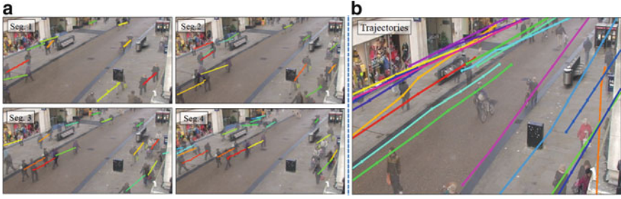
Fig. 4 (a) Tracklets found in four segments of a sample video sequence. (b) Tracklets are merged into full trajectories for all the pedestrians
