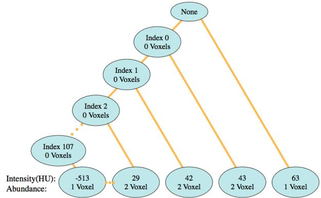
Fig. 2. An example of a tree of intensities for one region of interest; left nodes contain the height for simplistic indexing and easier calculations; right nodes contain the intensity value (in Hounsfield Units). Each node has a property, the abundance, or the number of voxels with that intensity.
